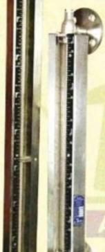
The "Taurus" make Tubular Level Indicator (Side Mounted). Indicator Top & Bottom liquid chamber is made from solid bar & IC Casting & Borosilicate Glass tube is fully protected by box section made out of thick M.S./S.S Channel. Economical design, heavy wall borosilicate glass tube 19mm OD available in single length up to 3 mtr., bolted gland with Tefion packing ensure positive leak tight.
